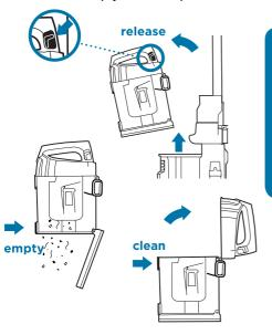
MAINTENANCE: Rinse pre-motor filters every 3 months, and HEPA filter once a year. Rinse with water only, and allow to air-dry completely before reinstalling.
