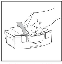
To avoid spills, be sure to hold the dust bin in an upright position. Pinch and lift to open the lid.
