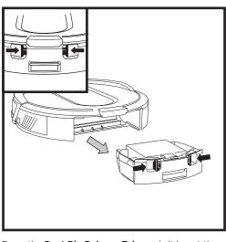
Press the **Dust Bin Release Tabs** and slide out the dust bin.
