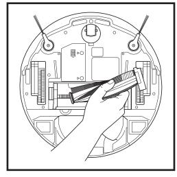
Lift out the brushroll, and clean off any debris. Reinstall the brushroll, inserting the flat end first. Close the brushroll access door and press down until both sides click into place.
