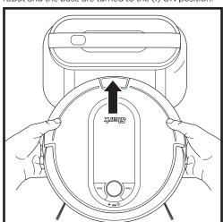
When the cleaning cycle is complete, or if the battery is running low, the robot will search for the base. If your robot doesn't return to the base, its charge may have run out. Make sure that all the protective film has been removed from the base, and recharge the robot
