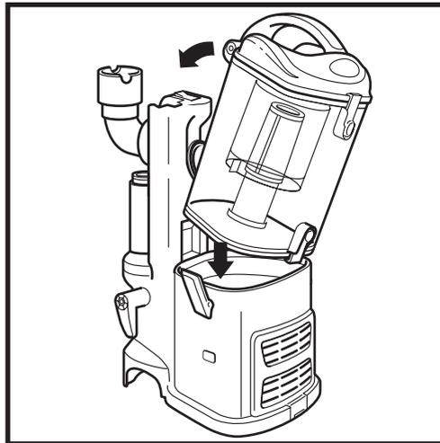
To reinstall, place the bottom of the dust cup into the pod and then tilt until it fits into place. Reattach side latches.
