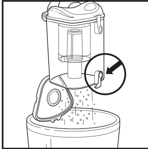
Hold the dust cup over a trash receptacle and press the door release button. Tap gently to empty. Press the door shut until it clicks into place.
