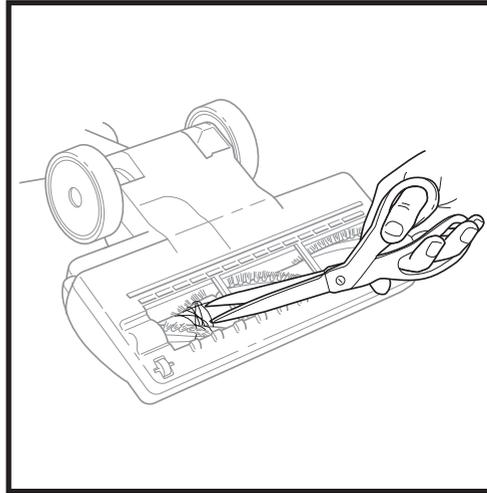
Inspect the airway and the brushroll. Remove any debris buildup. With scissors, carefully cut away any fibers or hair wrapped around the brushroll. Avoid damaging or cutting the bristles.
