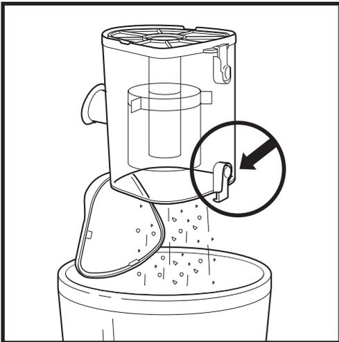
To remove debris from the **Lint Screen** in the dust cup, press the top release button and lift the handle to open. Gently brush debris off the screen.
