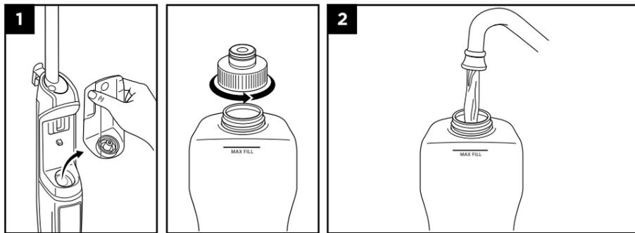
1. Pull out the clean water tank and unscrew the cap.
