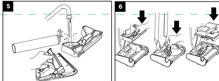
5. Wipe the inside of the nozzle clean of any leftover debris. Rinse off any leftover debris with tap water.
