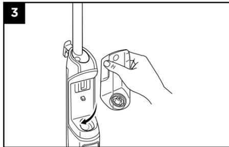
3. Screw on the cap. Reinstall the clean water tank into the unit until it clicks securely into place.
