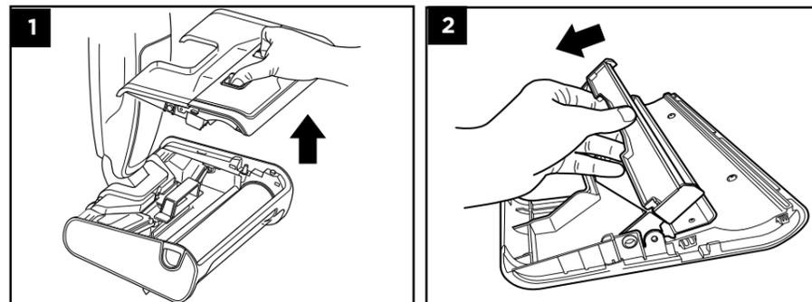
1. Remove the **Nozzle Cover**: Press both tabs and lift off the cover.
