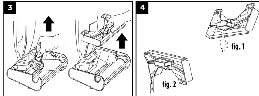
3. Remove the **Brushroll** and **Debris Tank**: Grip the side tab and lift out the brushroll, then remove the debris tank by pulling up on the handle.
