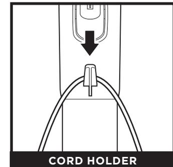
Use cord holder on the side of wand to hold cord in place while vacuuming.
