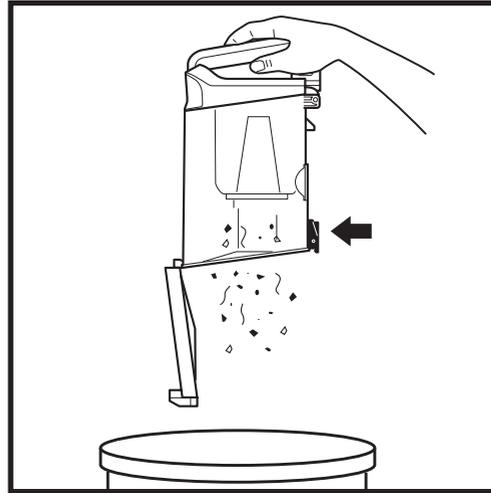
To empty debris into the trash, press the lower release button and the bottom of the dust cup will drop open.
