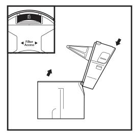
Hold the dust cup over the trash. Pull back on the yellow **Empty** button and pull up to open the dust cup lid until it clicks and locks in the open position. Gently tap the coneshaped screen inside the dust cup to knock dust and debris into the trash.
