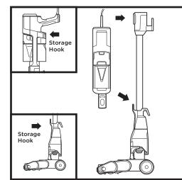
Press the **Wand Release** button near the top of the wand to detach the handheld vacuum. Align the **Catch** on the side of the handheld vacuum with the **Storage Hook** on the wand, then hang the handheld vacuum from the hook.
