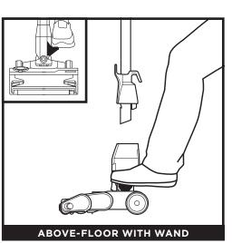
For more reach, detach the wand. Stand the vacuum upright, step on the **Foot Pedal** on the side of the nozzle, and pull up the wand to detach.
