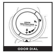
Flip up the dial handle and rotate the odor dial to adjust Odor Neutralizer Technology intensity or to unlock the dial for cartridge access.
