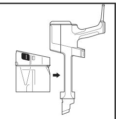
To reinstall, push the lid closed, then insert the dust cup into the handheld vacuum from the top, until it clicks into place.
