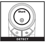
In Detect mode, Floor Detect technology automatically senses carpets and hard floors and adjusts the brushroll speed for optimal performance.
