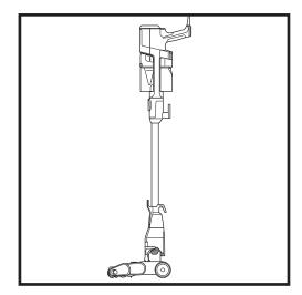
Wrap the cord around the two cord hooks. Start with the bottom hook and leave a little slack in the cord.
