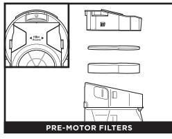
The **Pre-Motor Filters** should be rinsed every month. To remove the pre-motor filters, detach the dust cup, then slide down the Filter Access buttons on both sides of the dust cup lid. Pull out the filter housing, then lift out the **Foam Filter**. Next, remove the **Felt Filter** by the pull tab. After the filters have been rinsed and are completely dry, insert the foam filter into the housing first, then slide in the felt filter, and reinstall the housing into the dust cup lid.
