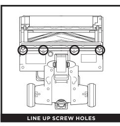
**2.** Align the 4 screw holes on the squeegee strip over the holes in the nozzle. Make sure the strip sits flush with the nozzle, then fasten it securely in place with the screws.
