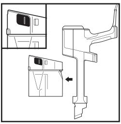
To remove the dust cup from the handheld vacuum, press the two **Dust Cup Release** buttons at the same time and pull out the dust cup from the top.
