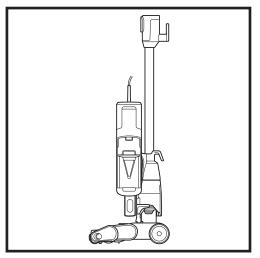
Wrap the cord around the two cord hooks. Start with the top hook, and leave a little slack in the cord.
