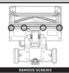
1. Turn the nozzle over and locate the squeegee bristle strip between the brushroll and the rear wheels. Use a Phillips-head screwdriver to remove the 4 screws.
