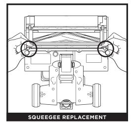
**1.** Hold the squeegee strip by the fabric flaps on the ends, with the bristle side facing up. Insert the plastic piece into the cavity first, while tilting the strip forward, toward the brushroll.
