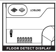
The Floor Detect display indicates which surface type has been detected.
