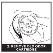
Rotate the cartridge counterclockwise in the dial housing and pull out the cartridge to remove it.
