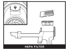
The **HEPA Filter** should be rinsed every 6 months. To remove the HEPA filter, detach the dust cup, then pull the **Filter Release** tab on the handheld vacuum filter cover. Remove the cover, then squeeze the side tabs on the HEPA filter and lift it out. After the filter has been rinsed and is completely dry, reinsert it into the handheld vacuum, then reattach the filter cover.
