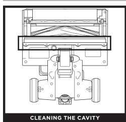
1. With the strip removed, clean the squeegee cavity and bristle strip. Use a paper towel to wipe off any debris or dust in the cavity and on the bristle strip.
