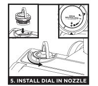
Align the teal arrow on the dial cover with the teal arrow on the nozzle, then reinsert the dial into the nozzle. Rotate the dial counterclockwise until it clicks into an intensity setting to engage. Rotate further to change the intensity setting.
