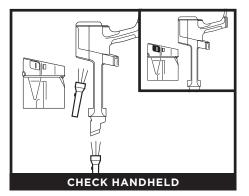
Remove the handheld vacuum from the wand and check all dust cup intake openings for debris or blockages.
