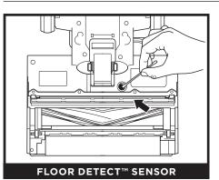
Make sure to clean the Detect sensors regularly, as hair and other debris may build up and obstruct them. If the sensors are partially obstructed, Detect mode will not function as expected.
