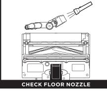
Detach the wand, turn the nozzle over, open the **Nozzle Hose Access,** and check for blockages.
