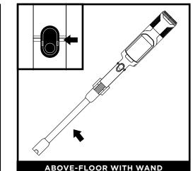
To detach the floor nozzle from the wand, step on the nozzle while pressing the nozzle release button at the bottom of the wand. Lift the wand to remove it. To reattach the wand, align it over the neck of the floor nozzle, then slide it on until it clicks into place.
