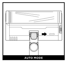
Automatically adjusts to different floor types, with brushroll speed optimized for deep carpet cleaning. When on bare floor, the indicator light on the nozzle will be BLUE. On carpet, the light will be MAGENTA. The light will turn RED if there is an error or clog. See Troubleshooting if this occurs.
