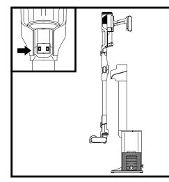
Place the vacuum on the dock with the wand in the cradle of the charging post. When the vacuum is properly docked, automatic evacuation will begin. The evacuation cycle will last for 15 seconds.
