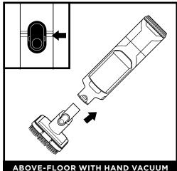
Detach the hand vacuum to clean abovefloor areas. Press the front latch release button on the hand vac where it meets the wand, then lift off the hand vacuum. To attach an accessory to the hand vacuum, slide it into the opening in the nozzle. To remove, press the release button and slide out the accessory.
