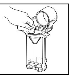
To deep-clean the dust cup, slide the release button until the lid opens completely. Wipe away any dust and debris with a dry cloth, then rinse it out with water. Use a damp cloth to remove any remaining debris. Allow the dust cup to air-dry completely for at least 24 hours before reinstalling it.
