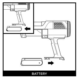
To remove the battery from the hand vacuum, press the release tab on the battery cap and slide out the battery. To reinstall, slide the battery into the compartment in the handle until it clicks into place.
