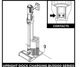
Charge the unit by placing it on the dock. Make sure the contacts on the wand are aligned with the contacts on the charging post. When charging is complete and you need to use the unit again, lift it off the dock.
