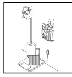
The dock dust bin holds up to 30 days' worth of dust and debris. To remove the bin, press the dust bin release button and lift the bin out by the handle.
