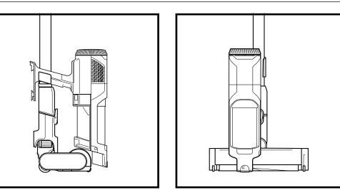
For quick and easy short-term storage, attach the hand vacuum to the wand by placing it onto the pre-assembled wand storage clip.
