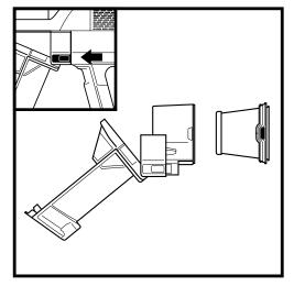
With the dust cup open and the power off, press both release buttons and slide the dust cup out of the hand vac.
