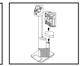
To access the Auto-Empty Exhaust Foam Filter, remove the dust bin. Before removing the Exhaust Foam Filter, vacuum off any fine debris from the surface. Lift the Exhaust Foam Filter out of the dock, then rinse it with water only (do not use soap). Allow the filter to air-dry completely before reinstalling it.
