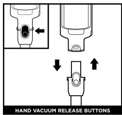
To detach the hand vacuum from the wand, press the front latch release button on the hand vac where it meets the wand, then lift off the hand vacuum. To reattach the hand vacuum to the wand, align the hand vacuum opening over the top of the wand and slide it on until it clicks into place.
