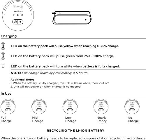
When the Shark' Li-ion battery needs to be replaced, dispose of it or recycle it in accordance with local ordinances or regulations. In some areas, it is illegal to place spent lithium-ion batteries in the trash or in a municipal solid waste stream. Return spent batteries to an authorized recycling center or to the retailer for recycling. Contact your local recycling center for information on where to drop off the spent battery.
