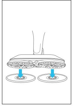
2. To attach the Dirt Grip Soft Scrub Pads, place BOTH pads flat on the floor with plastic rings facing up. Align the unit directly over the plastic rings on the pads. Gently lower the Mop Head onto the pads, pressing until the pads are secure.
