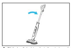
**3.** Tilt the handle back to activate the spinning pads and begin scrubbing.
