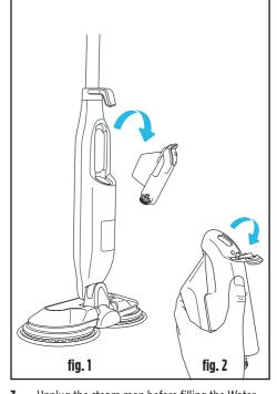
3. Unplug the steam mop before filling the Water Tank. To remove the tank, pull it out, away from the mop body (fig. 1). Pull the top rubber fill cap back and with cold or normal temperature WATER ONLY (fig. 2).
