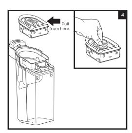
**4.** Clean the filter housing and the foam filter after every use. Pull out the foam filter and hand-wash with warm water and soap.
