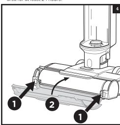
**4.** To reinstall the brushroll cover, insert the tabs on the cover into the slots on the nozzle. Press down on the cover until it clicks into place.
