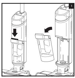
1. To remove the dirty water tank, press the release button and pull out the tank.
