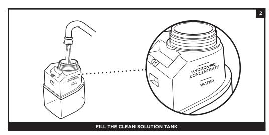
Unscrew the cap and add water to the tank, up to the WATER line. Next, add Shark HydroVac $^{\text{TM}}$  Multi-Surface Concentrate, filling to the HYDROVAC CONCENTRATE line. Replace the cap and reinsert the tank until it clicks into place. The top of the tank should be flush with the top of the body.
