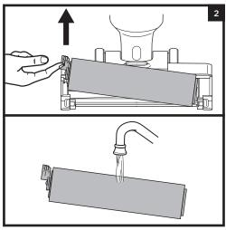
Remove the brushroll by pulling up on the pull tab on the left side of the nozzle. Wipe away any debris stuck on the back wall.
