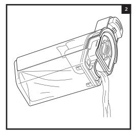
To dispose of liquid waste only, pour it out though the Easy Pour spout on the back of the dirty water tank
