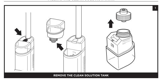
Press the release button and lift off the Clean Solution Tank.
