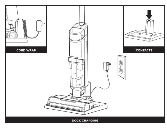
Charge the unit by placing it on the dock. Make sure the contacts on the body are aligned with the contacts on the charging dock.
