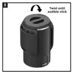
**3.** With the HEPA filter reinstalled, twist the filter door clockwise until it clicks into place.
