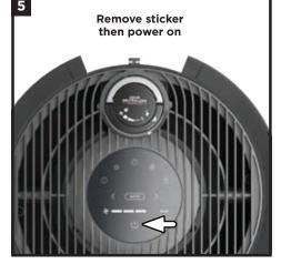
**5.** Carefully remove the yellow sticker on the top of the product to access the control panel.
