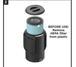
**2.** Take the HEPA filter out of its plastic packaging. Reinstall the HEPA filter in either orientation.
