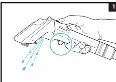
1. Before storing, follow Maintenance and Cleaning Instructions above. Be sure to release all pressure from the hand tool by placing it over a sink or toilet and pressing the spray trigger until all liquid has been released. Lay out all attachments to dry.
