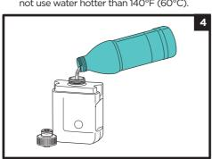
4. Lift StainStriker Tank by its sides to remove it, and fill with Shark OXY Multiplier. Replace the cap and tighten it.
