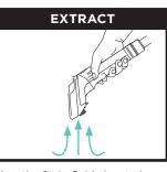
For Wet Stains, follow the Stain Guide located on the hand tool. Turn ON using the power button and vacuum up the liquid mess. Spray the stain area. Scrub stain with the bristles, then tilt hand tool forward and drag across stain area to extract liquid. Repeat if needed. To avoid longer dry times, do not over spray.
