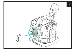
tool on the unit. Wrap the hose around the base of the unit and store the hand tool in its holder.
