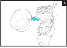
Be sure to rinse the Pet Mess Tool, cover, rubber bristles mesh filter, and cup with soap and water. Allow all parts to air-dry completely before reassembling. Make sure the filter clicks into place and to rotate the cup to the locked position before use.
