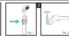
2. Remove the hand tool from the hose by pressing the Detach Button (fig. 1). To clean the airpath in the tool, open the cover (fig. 2). Aim the hand tool into a sink or toilet and press the spray trigger to release remaining pressure.
