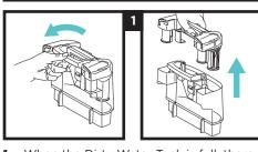
1. When the Dirty Water Tank is full, there will be a change in sound as the float valve closes. Switch off the unit and detach the tank, making sure to keep it upright to prevent spills. Pull the handle back, then lift off the lid. Pour out the contents into a sink or toilet.
