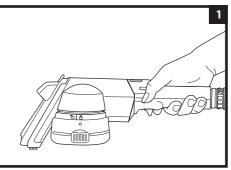
The Pet Mess Tool is designed to tackle pet messes while keeping debris and liquid out o the interior of the Spot Cleaner (Pet Mess Tool not included with some units. To order tools, visit sharkaccessories.com. To use the Pet Mess Tool, attach it to the Crevice Tool, then spray, scrub gently to prevent squashing in cup, and extract pet stains and messes. Keep the cup on the Pet Mess Tool upright to avoid spillage
